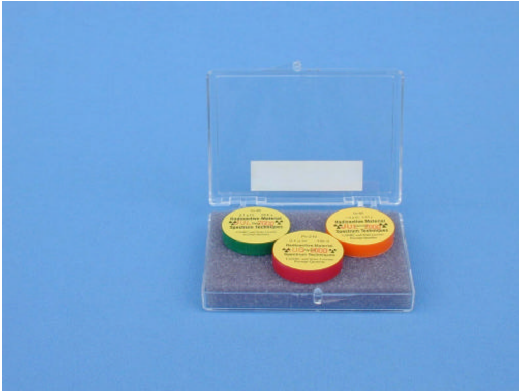
Figure 2 – Kit with one each of an alpha emitter, beta emitter, and gamma emitter
