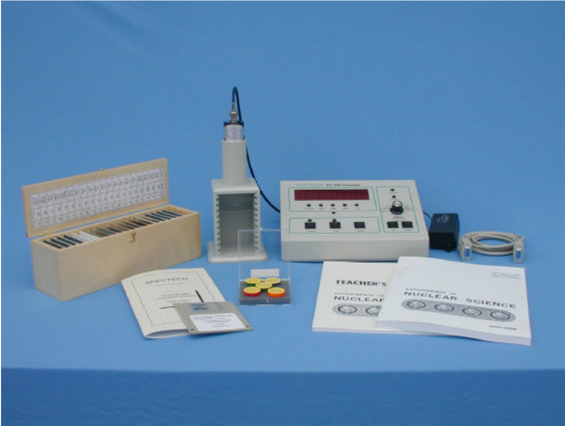
Figure 2: ST350 setup with sources and absorber kit.
