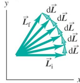
In the case of the spinning gyroscope we observe the axis of the gyroscope (or the angular momentum vector  $\vec{L}$ ) rotating about the pivot point. This peculiar motion is called *precession*. The **precession angular speed** is denoted by the quantity  $\Omega$ :
