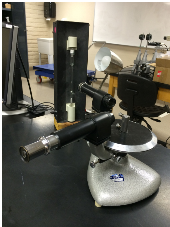
FIG. 1. The spectroscopy experiment is shown in the figure above. A glass tube containing a rarified gas is mounted in the vertical HV apparatus. When the discharge tube is turned on, light passes through a collimator (seen facing the tube), and goes to the diffraction grating (not shown), and then bent toward the telescope where the observer makes the measurement (the diffraction angle, \theta ).
