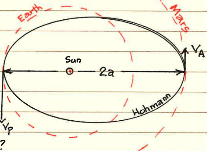
What are the values for  $V_A$  and  $V_p$  for the elliptical Hohmann transfer orbit?
