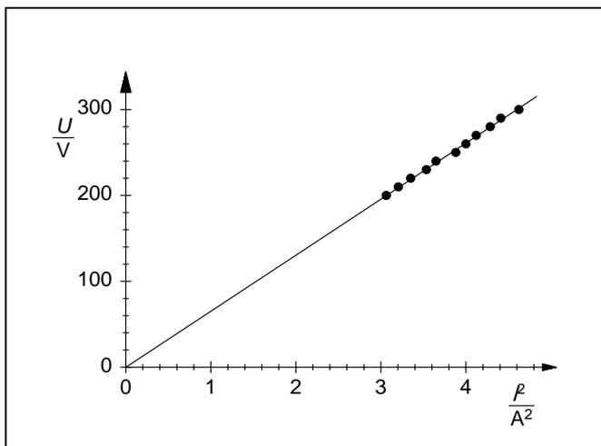
**Determination of the proportionality factor  $k$  from the calibration of the Helmholtz magnetic field:**
