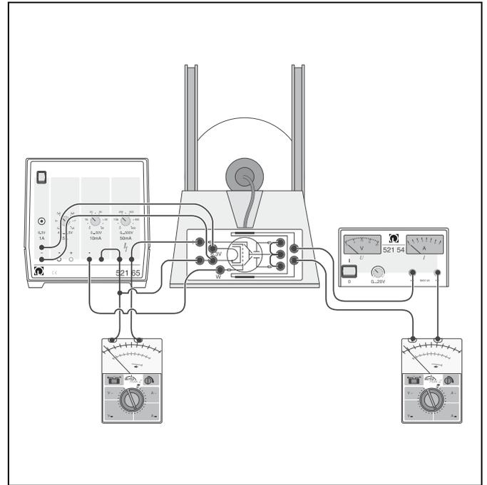
Fig. 3 Electric connection
