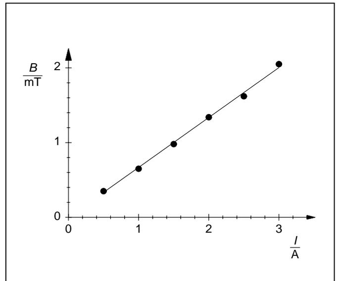
Fig. 7 Calibration curve for the magnetic field of the Helmholtz coils
