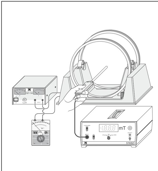
Fig. 5 Set-up for calibration of the Helmholtz magnetic field
