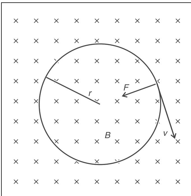
Fig. 1 Deflection of electrons in a magnetic field  $B$  by the Lorentz-force  $F$  into a circular orbit of a given radius  $r$ .
