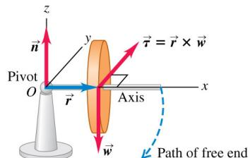
When the flywheel is not rotating, its weight creates a torque around the pivot, causing it to fall along a circular path until its axis rests on the table surface.
