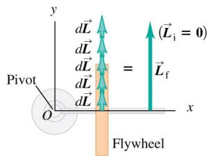
In falling, the flywheel rotates about the pivot and thus acquires an angular momentum  $\vec{L}$ . The direction of  $\vec{L}$  stays constant.
