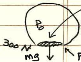
$$\text{Net force} = (P - P_0)A - mg = (3.028 \times 10^5 \text{ Pa})(0.75 \text{ m}^2) - 300 \text{ N}$$
