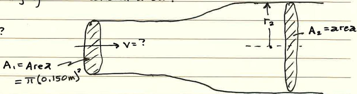
$$\text{Volume Rate} = R = A_1 v_1 \quad v_1 = \frac{R}{A_1} = \frac{1.20 \text{ m}^3/\text{s}}{\pi(0.150\text{m})^2} = \underline{\underline{16.98 \text{ m/s}}}$$
