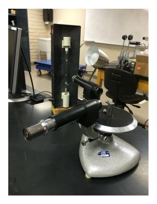
FIG. 1. The spectroscopy experiment is shown in the figure above. A glass tube containing a rarified gas is mounted in the vertical HV apparatus. When the discharge tube is turned on, light passes through a collimator (seen facing the tube), and goes to the diffraction grating (not shown), and then bent toward the telescope where the observer makes the measurement (the diffraction angle,  $\theta$ ).
