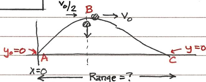
$$\text{Eq. 3} \quad y = v_{oy} t - \frac{1}{2} g t^2 \quad 0 = v_{oy} t - \frac{1}{2} g t^2$$
