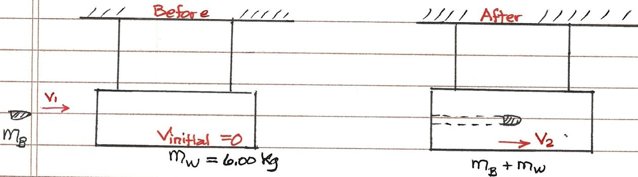
$$P_{\text{initial}}^{\text{Total}} = P_{\text{final}}^{\text{Total}} \quad m_B v_1 = (m_B + m_W) v_2$$
