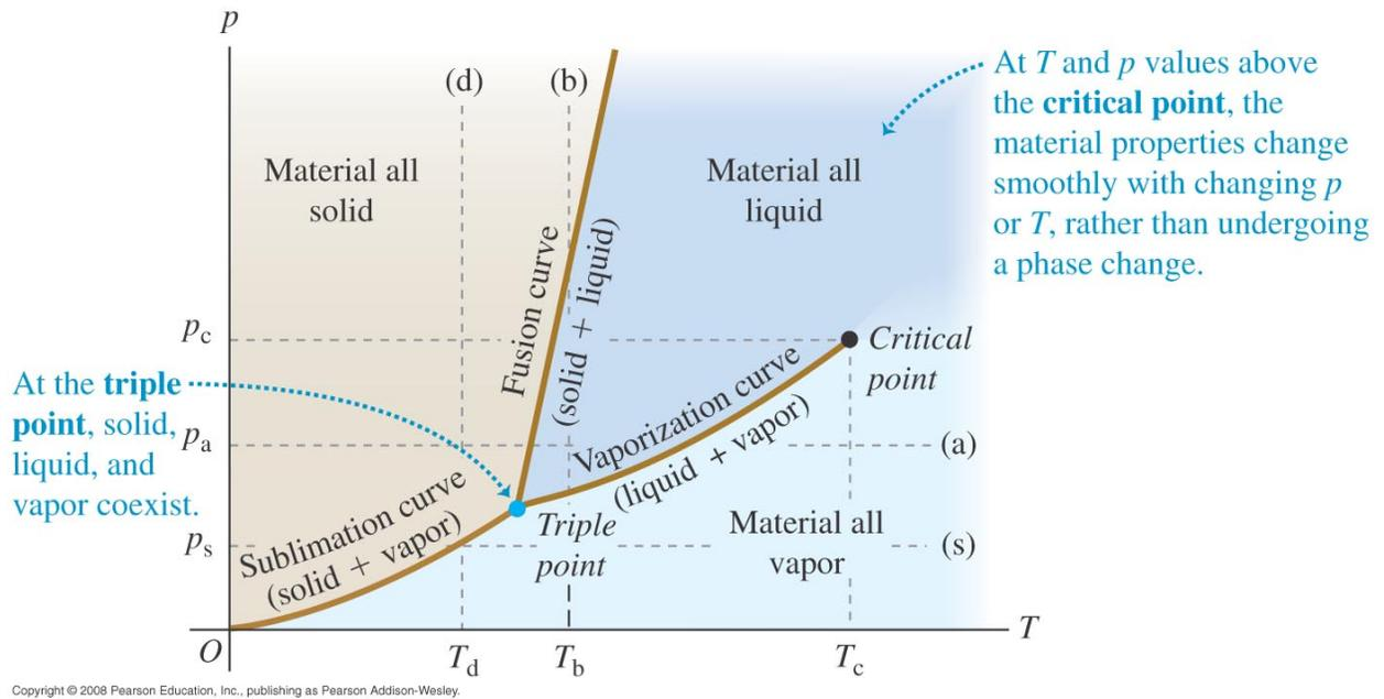
Figure 3: A typical  $p$ - $T$  diagram depicting the phase transitions for most materials. Beyond the “critical point” the substance is referred to as a **supercritical fluid**. There is no longer a phase transition between vapor and liquid. This is where the liquid and gaseous phases of the substance merge into a single phase, and where distinct liquid and gas phases do not exist. The supercritical fluid can effuse through solids like a gas, and dissolve materials like a liquid.
