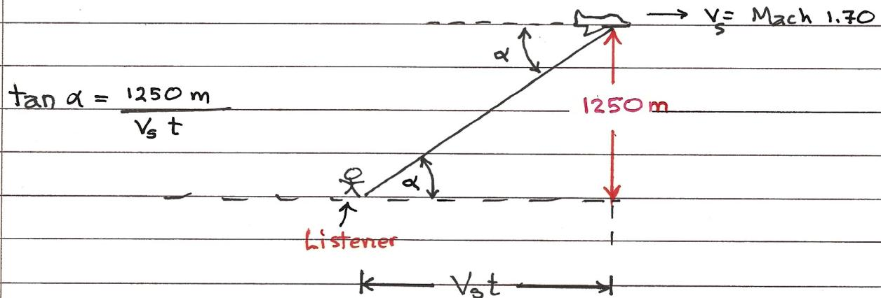
$$t = \frac{1250 \text{ m}}{v_s \tan \alpha} = \frac{1250 \text{ m}}{1.70 (344 \text{ m/s}) \tan 36.0^\circ} = 2.94 \text{ s}$$
