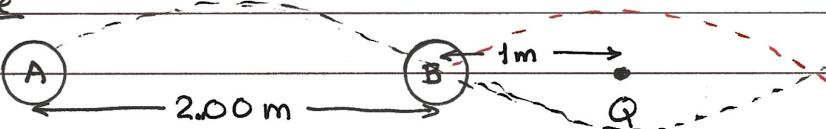
$$2.00 \text{ m} = n \frac{\lambda}{2} \quad \text{for destructive interference.}$$
